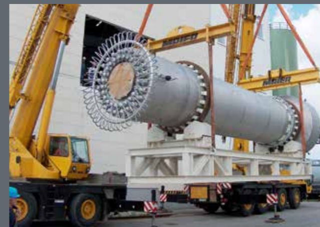
Indirect rotary tube with on-board heat exchanger
