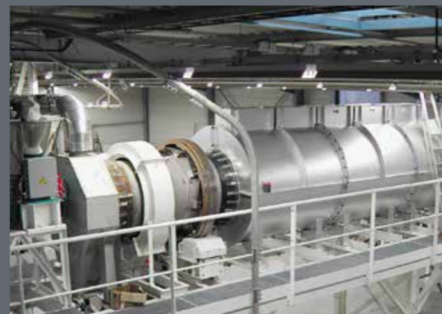
Indirect rotary tube heated through the shell
